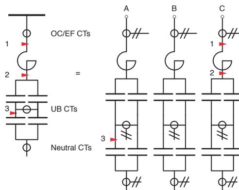
The unbalance CTs are generally required to register very low unbalance current, with trip levels in the range of 200 mA. CTs with good accuracy in the lower current ranges are therefore required. In the case of a typical 330 kV 160 Mvar capacitor bank with damping reactors of 11 mH and a network fault level of 50 kA, a typical line side CT specification will be 500:1 A, 10P20 5 VA, for the same physical layout as earlier.
